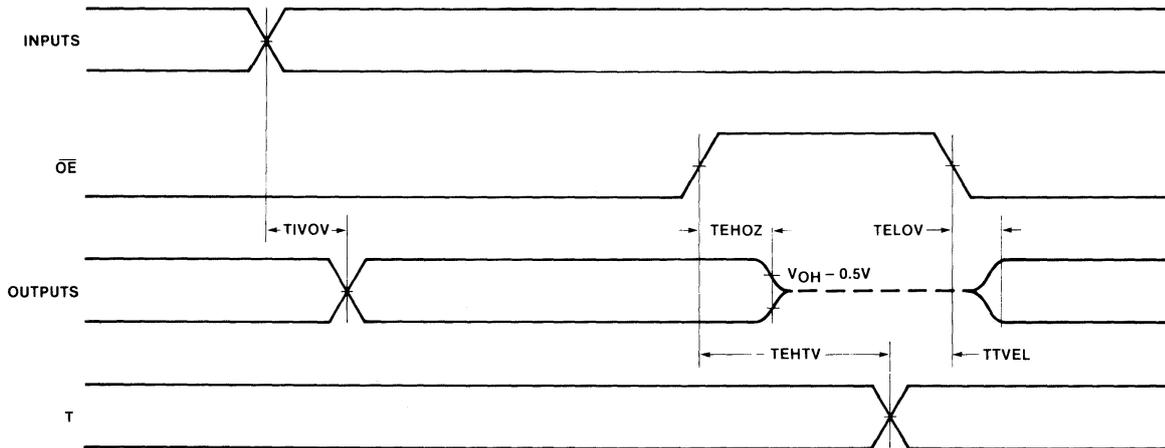
**NOTE:** 1. ALL TIMING MEASUREMENTS ARE MADE AT 1.5V UNLESS OTHERWISE NOTED.
