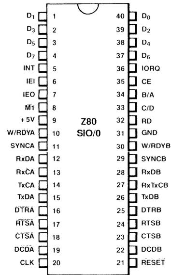
Figure 6. 40-pin Dual-In-Line Package (DIP), Pin Assignments
