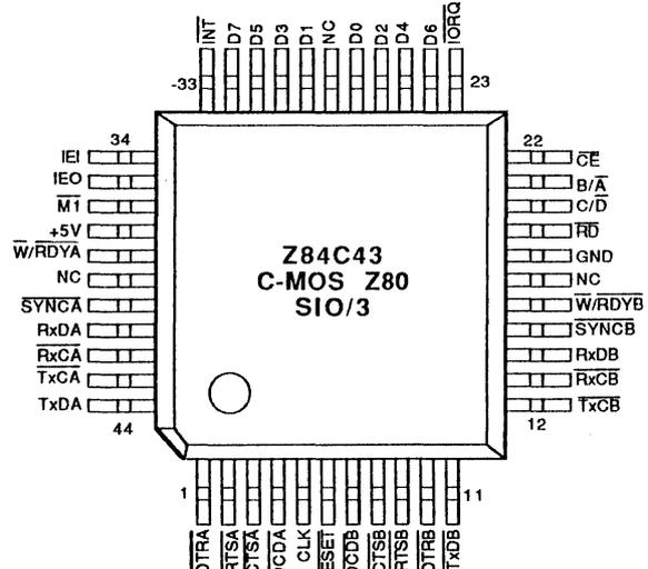
Figure 7b. 44-pin Quad Flat Pack Pin Assignments
