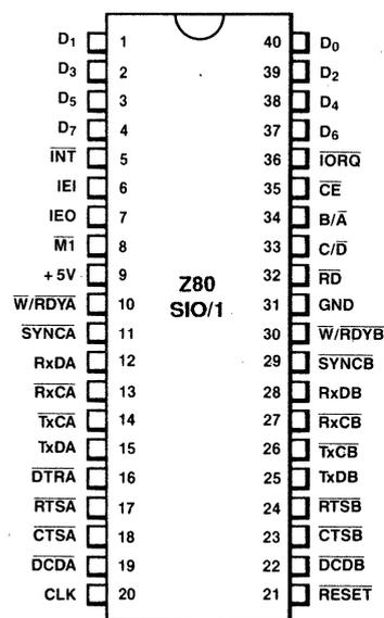
Figure 4. 40-pin Dual-In-Line Package (DIP), Pin Assignments
