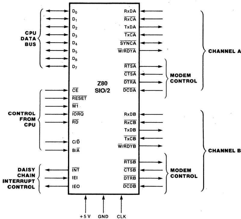
Figure 1. Pin Functions
