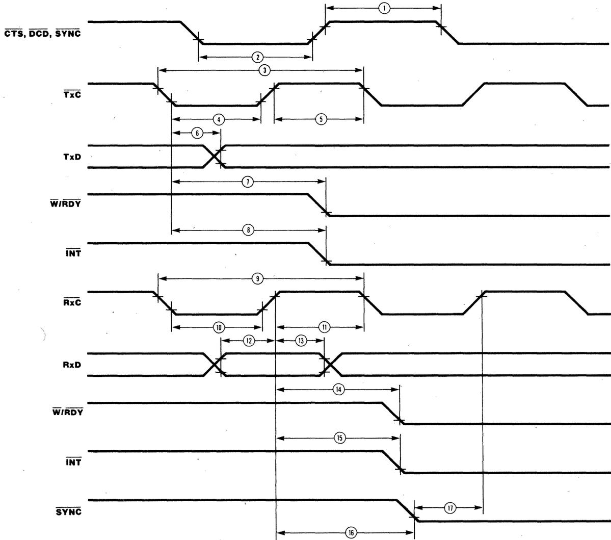
**AC CHARACTERISTICS TIMING (Z844X / NMOS Z80 SIO)**
