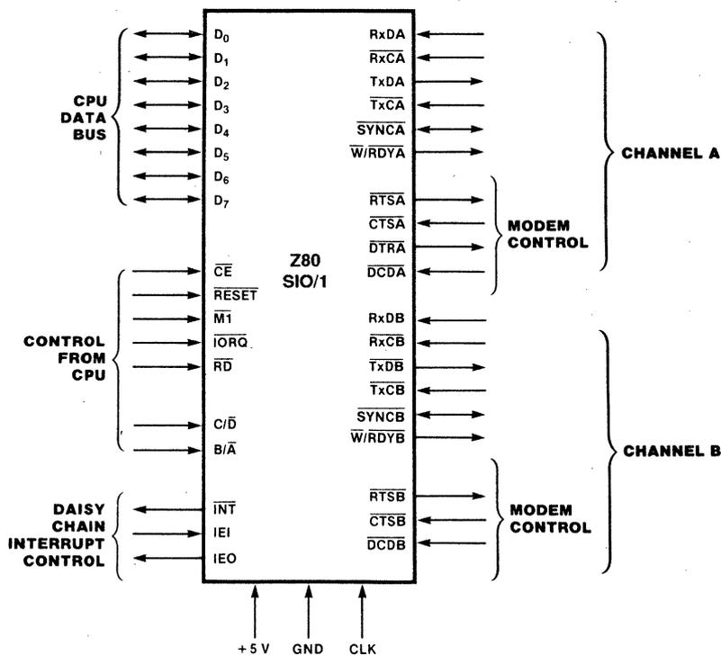
Figure 3. Pin Functions
