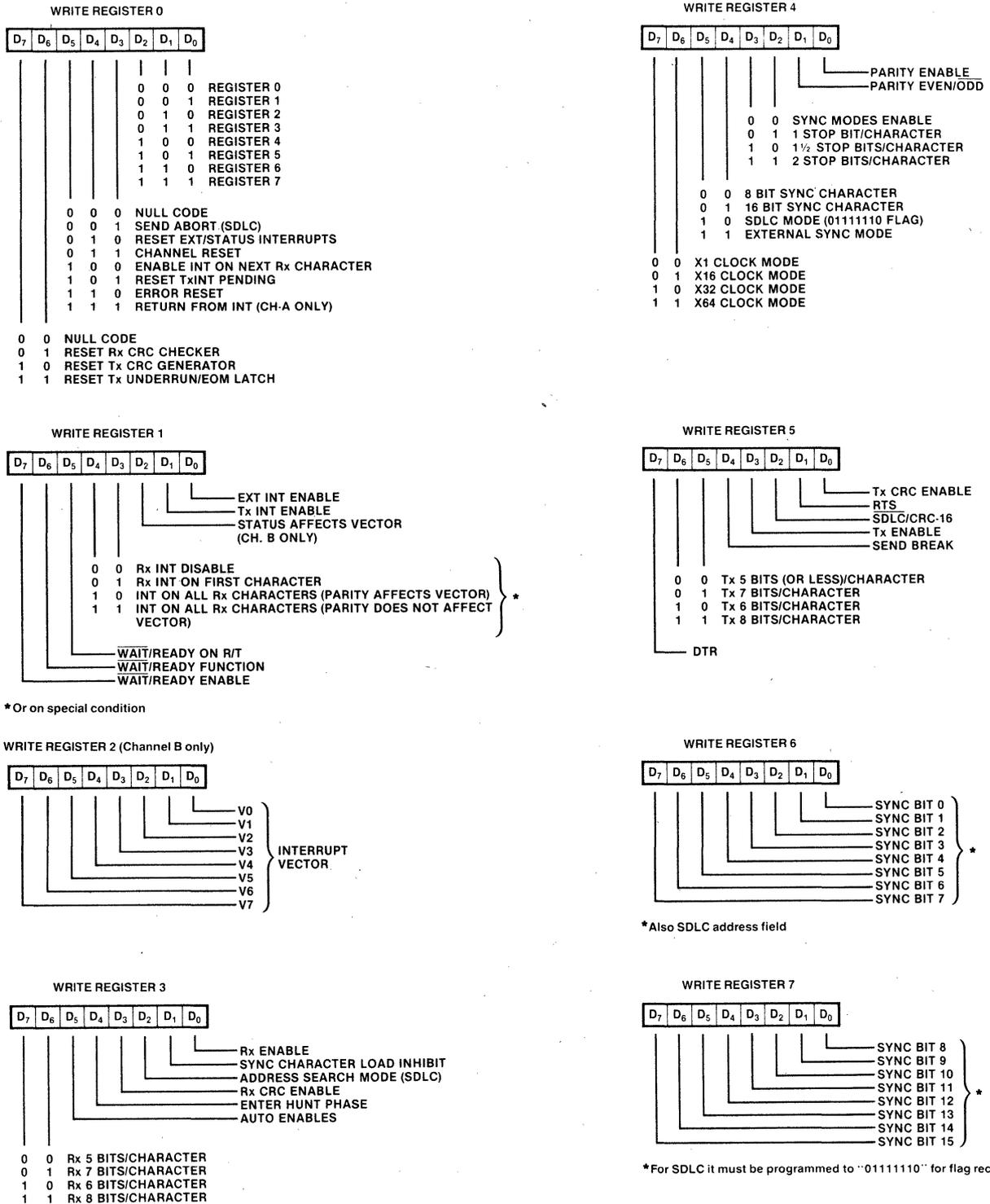
**Figure 14. Write Register Bit Functions**
