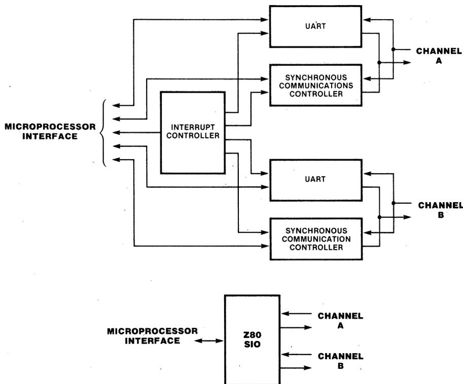
Figure 9. Conventional Devices Replaced by the Z80 SIO
