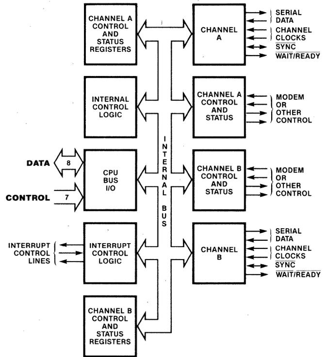
Figure 8. Block Diagram
