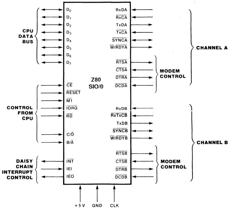
Figure 5. Pin Functions
