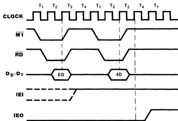
Figure 18. Return from Interrupt Cycle
