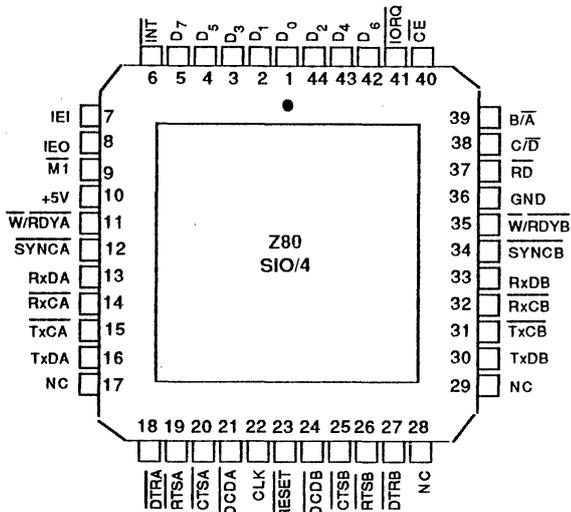
Figure 7a. 44-pin Chip Carrier, Pin Assignments
