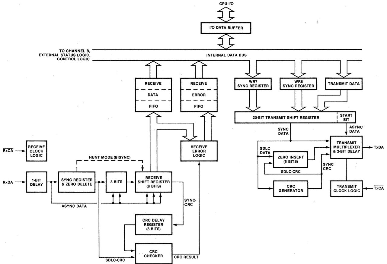
Figure 12. Transmit and Receive Data Path (Channel A)
