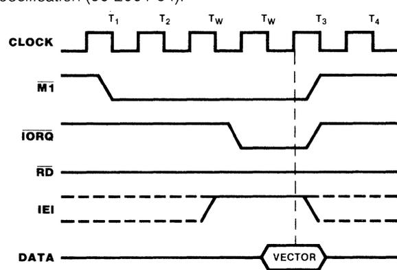
Figure 17. Interrupt Acknowledge Cycle
