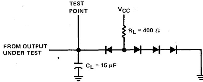
$C_L$  includes probe and jig capacitance.
